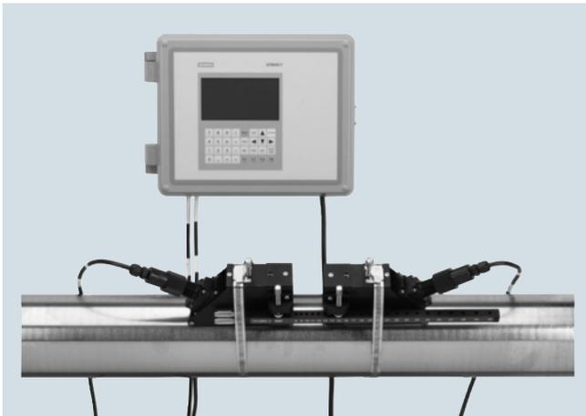
SITRANS FUS1010 is the most versatile clamp-on ultrasonic flow display transmitter available today. It can operate in either Wide-Beam Transit time or Reflexor (Doppler) mode, making it suitable for virtually any liquid, even those with high aeration or suspended solids.
